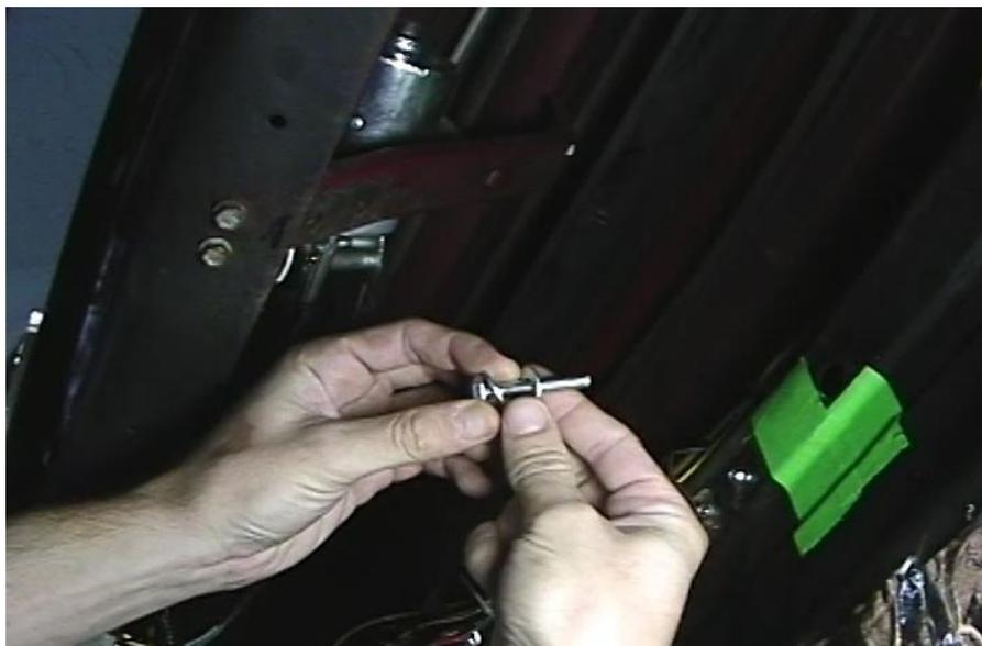
Note: Cowl Vent tab should be captured between the two washers, one on each side of vent tab.
