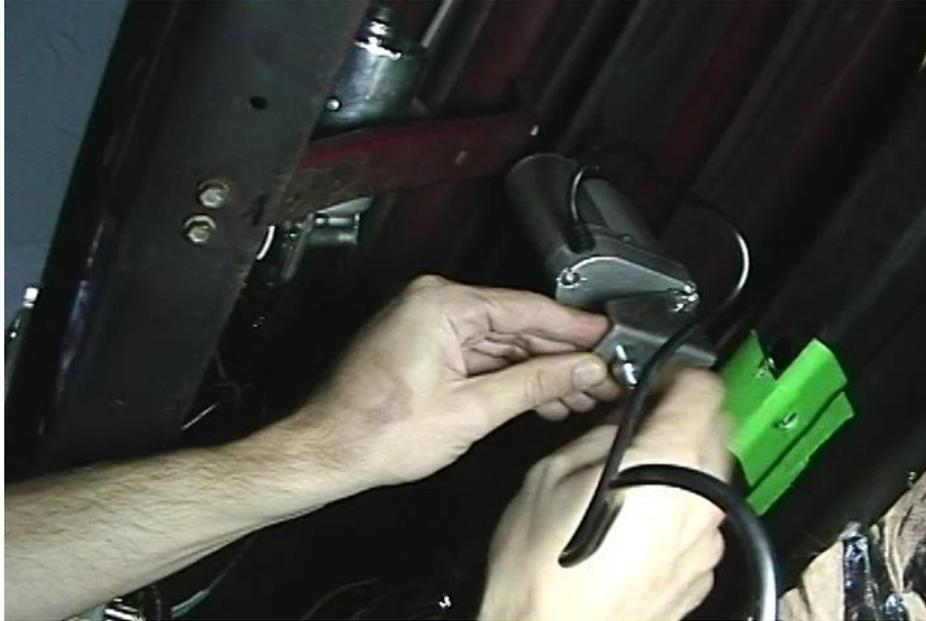
Note: The bottom hole of the Mounting Bracket has two nuts to compensate for the ledge on firewall.
